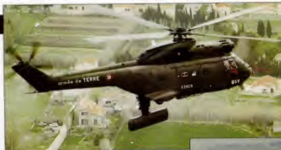
Left: The French Orchidée battlefield surveillance radar program was shelved in 1990, but was revived during Operation Desert Storm. The system was carried aboard a Puma.
